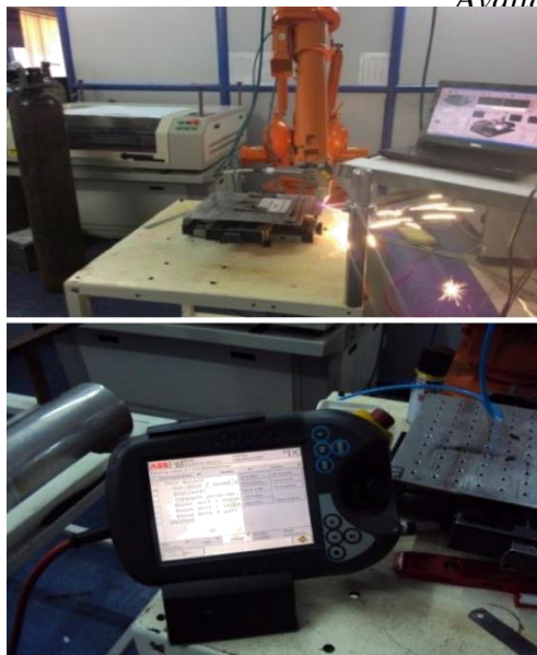
Fig1 Photographic view of laser beam micro machining system
