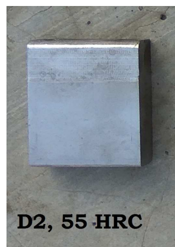
Fig. 2. Punch made by D2 material having hardness of about 55 HRC initially
