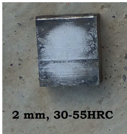
Fig. 3. Punch made by EN19 material having hardness of about 30 HRC initially and then induction hardened up to 55 HRC and 2mm depth
