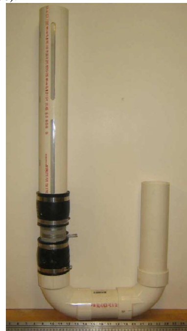
Fig. 1: Falling head permeameter used for 7.62 cm (3") diameter porous concrete specimens
