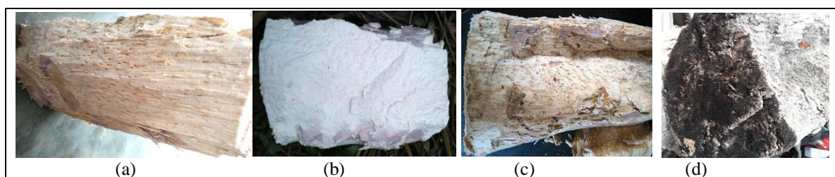
Fig. 2. Sago Piths Textures and Color Changes over Time due to Oxidation Process
