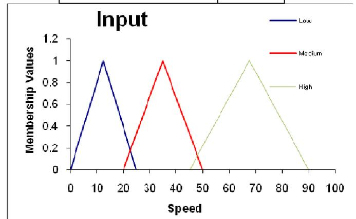
Fig. 2 Plot of membership function for input variable “Speed”
