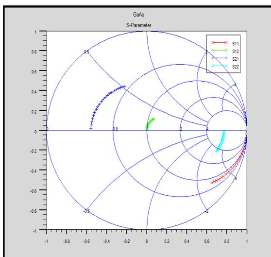
Fig.24 S-Parameter of GaAs MOSFET in TCAD
