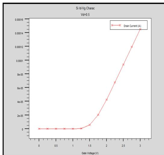
Fig: 15. Id-Vg Characteristics of Si MOSFET  $V_d=0.5\text{V}$
