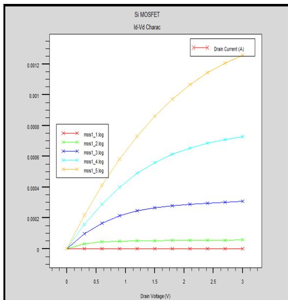
Fig: 12. Id-Vd Characteristics of Si MOSFET
