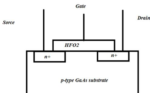
Fig.5: Basic structure of n-MOSFET
