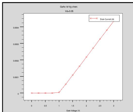
Fig: 20. Id-Vg Characteristics GaAs MOSFET for  $V_d=0.05\text{V}$
