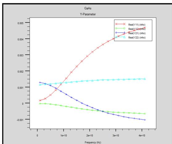
Fig. 23 Y- Parameter of GaAs MOSFET in TCAD
