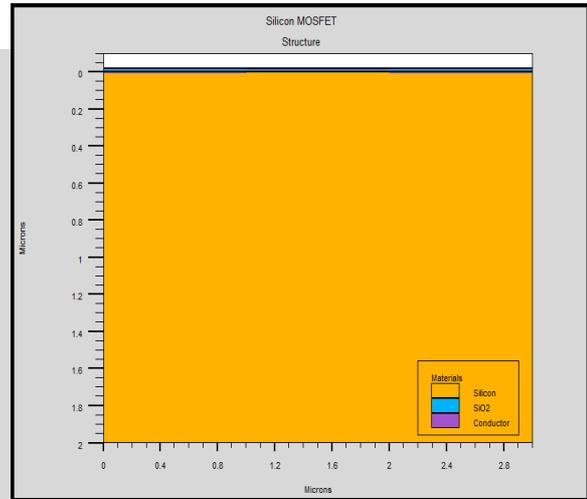
Fig: 9. Si MOSFET structure in TCAD of  $L_g=1\mu\text{m}$ .
