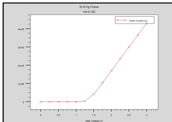
Fig: 14. Id-Vg for Si MOSFET  $V_d = 0.125\text{V}$
