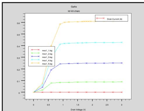
Fig: 19. Id-Vd Characteristics of GaAs MOSFET
