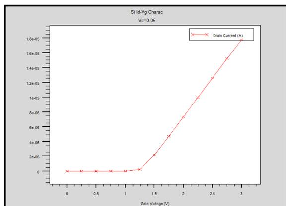
Fig: 13. Id-Vg for Si MOSFET  $V_d = 0.05\text{V}$
