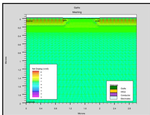
Fig: 18. GaAs MOSFET Meshing Structure
