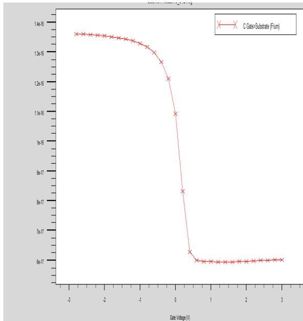
Fig: 8. C-V Characteristics of MOS Capacitor structure
