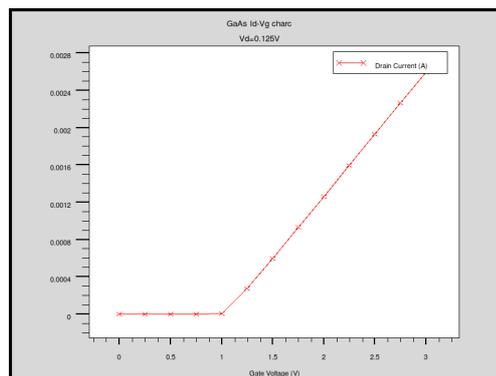
Fig: 21. Id-Vg Characteristics of GaAs MOSFET  $V_d=0.125\text{V}$
