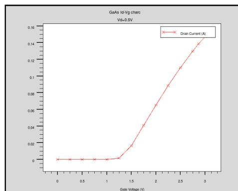
Fig: 22. Id-Vg Characteristics of GaAs MOSFET  $V_d=0.5\text{V}$
