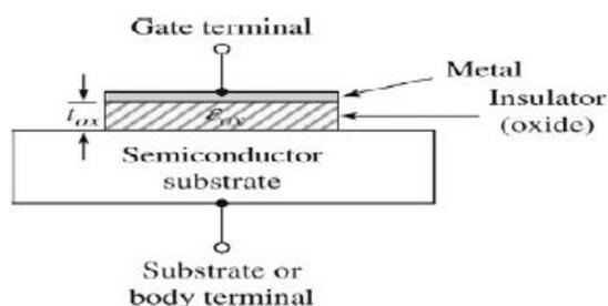
Fig.1: Basic MOS capacitance structure
