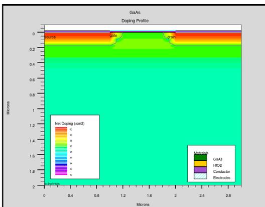
Fig: 17. GaAs MOSFET Structure with Net doping
