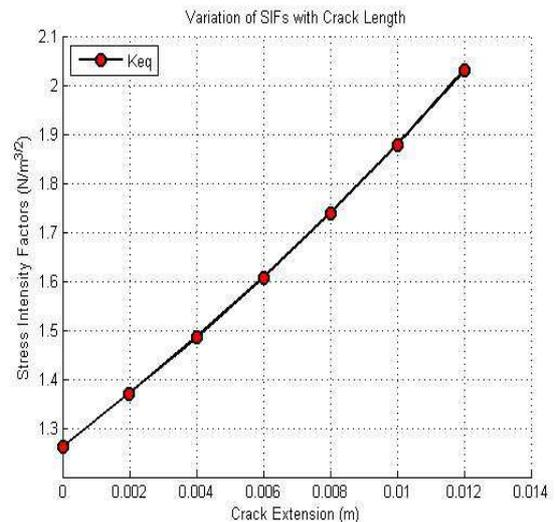
During combined loading of edge crack rectangular body, **Fig. 2(a)** shows the variation of stress  $\sigma_{yy}$  acting along the y-direction during the 1<sup>st</sup> step. The maximum stress obtained is near about 30 MPa near the crack tip. **Fig. 2(b)** shows variation of stress intensity factor  $K_{eq}$  for Edge crack with crack extension in combined loading. In this case also the crack extends by near about 0.012m before the ultimate fracture of the rectangular body.
