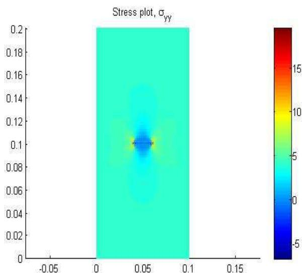
**Fig. 3(a)** Stress plot of  $\sigma_{yy}$  (MPa) during Combined loading
