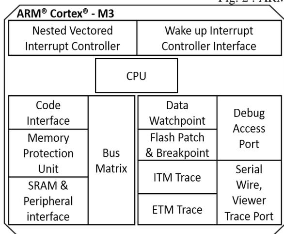
Fig. 3 ARM Cortex-M3 chip diagram
