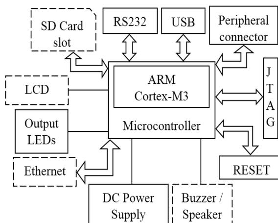
Fig. 1 : General block diagram of breakout board
