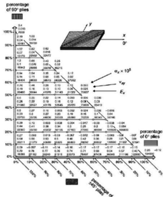
Fig. 2: Young's Modulus( $E_x$  in MPa), Poisson's ratio ( $\nu_{xy}$ ) and Co-efficient of thermal expansion ( $\alpha$ ) as functions of ply percentages for Carbon / Epoxy Laminate ( $V_f = 60\%$ ; Ply thickness = 0.13 mm) [12]
