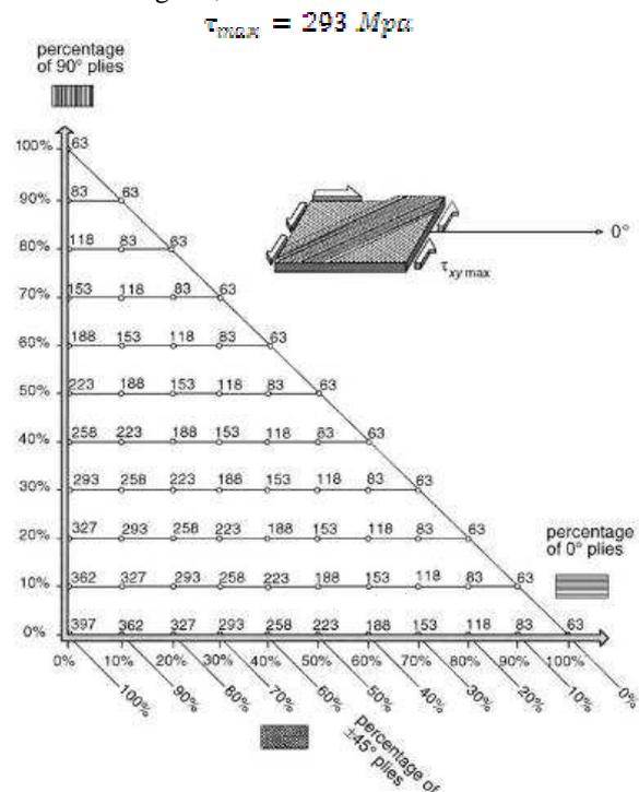
Fig.1: Maximum shear stress ( $\tau_{max}$ ) as a function of ply percentages for Carbon/Epoxy Laminate ( $V_f = 60\%$ ; Ply thickness = 0.13 mm)[12] Consider factor of safety as 6.
