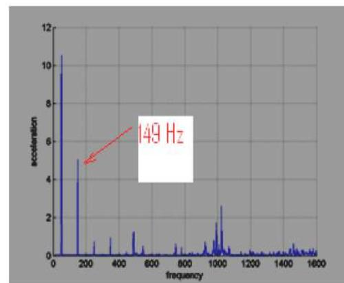
Figure 4 Outer race fault[1]
