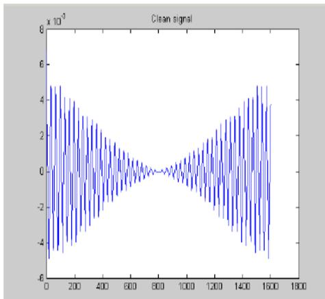
Figure 5 Time domain signal for healthy bearing[1]
