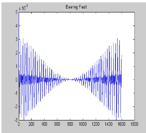
Figure 6 Time domain signal for faulty bearing[1]
