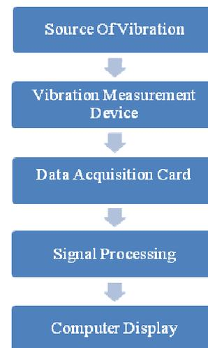
Figure: 1 Component of Architecture[8]
