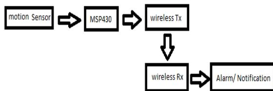
Fig. 4: Block Diagram of the system.
