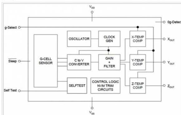
Fig. 2: Internal block diagram of the sensor.
