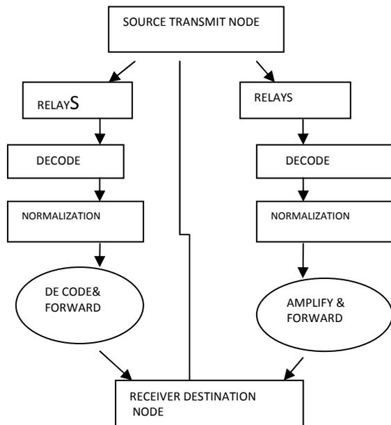
Fig. 5: Transmit Diversity and Relay Selection Algorithm
