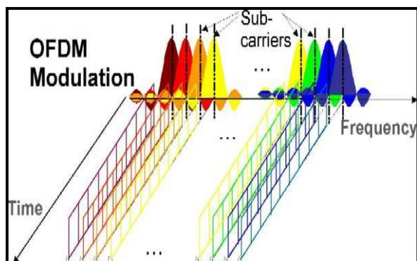
Fig. 3: Diagram of OFDM
