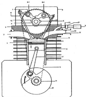
**THIRD STROKE (1<sup>ST</sup> POWER OR EXPANSION STROKE):-**
