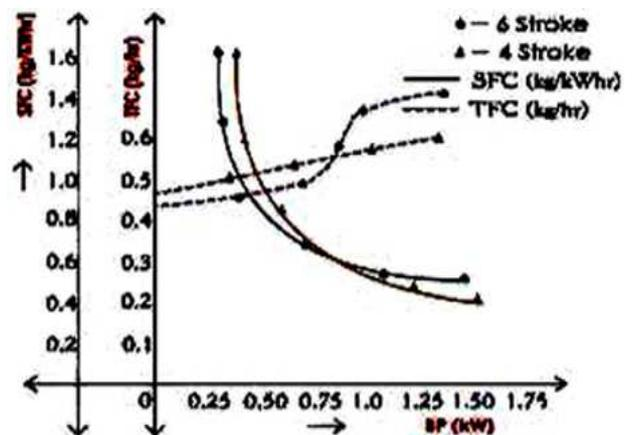
Graph-1: Bp Vs TFC & SFC at 320rpm
