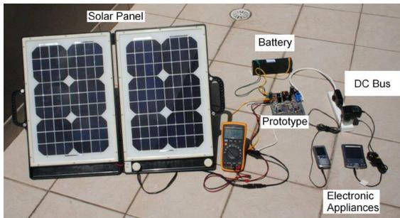
Fig.1: Hardware implementation of the proposed dc bus system with common portable electronics devices [2].
