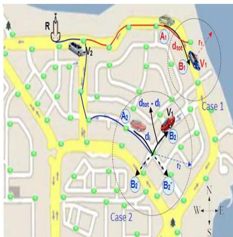
**Fig. 6. Sending a packet from an RSU to a vehicle:
