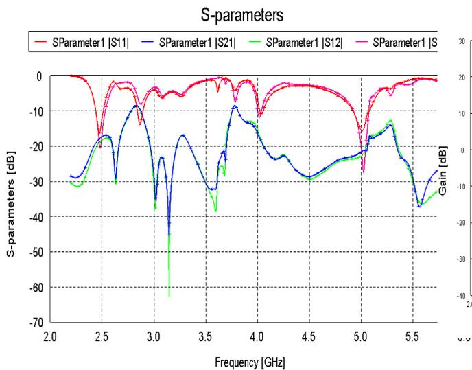
Fig. 3. Simulated S-parameter after introducing parasitic element.
