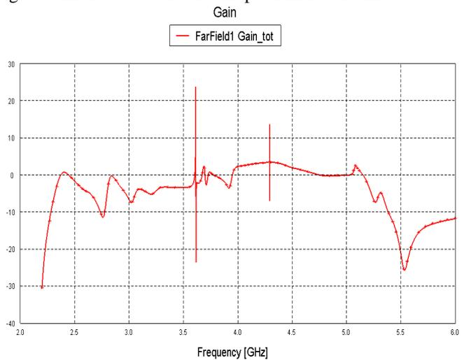
Fig. 5. Total Gain of 4-shaped MIMO antenna.
