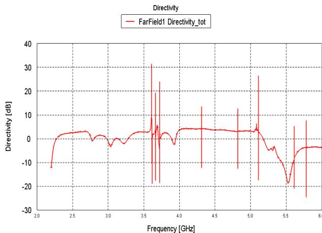
Fig. 7. Directivity of an antenna
