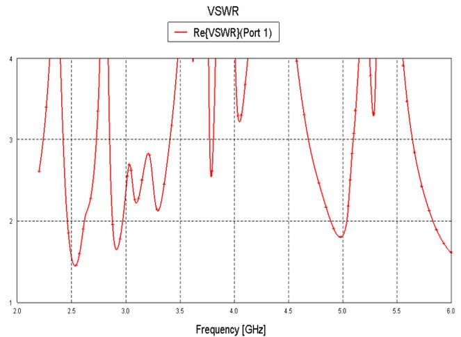
Fig. 4. Simulated VSWR of 4-shaped MIMO antenna.
