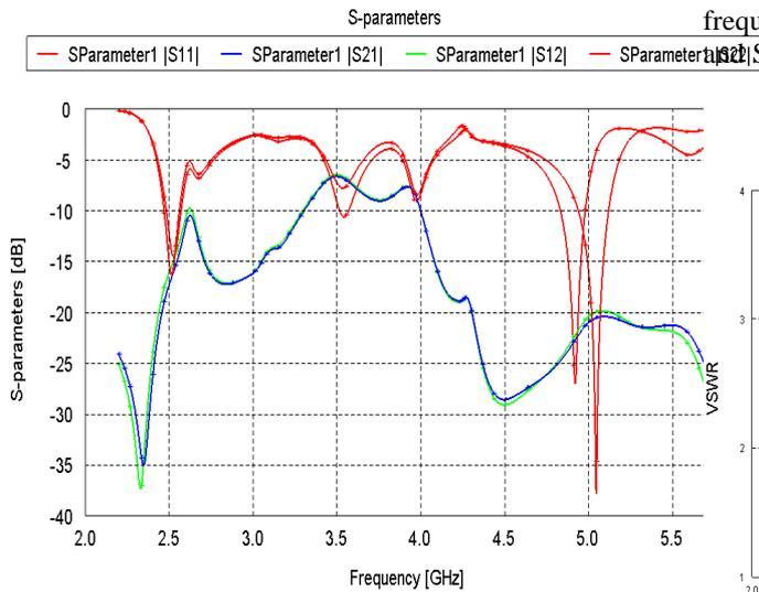
Fig. 2. Simulated S-parameter before introducing parasitic element.
