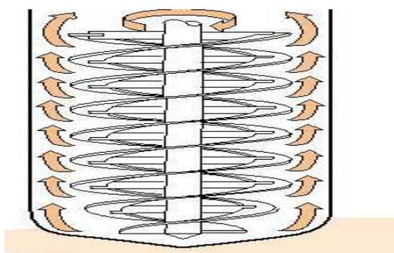
Fig. 6: Helical Impeller
