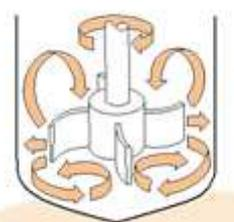
Fig. 5: Curved blade turbine
