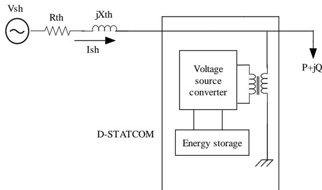
Fig. 11. Block Diagram of STATCOM
