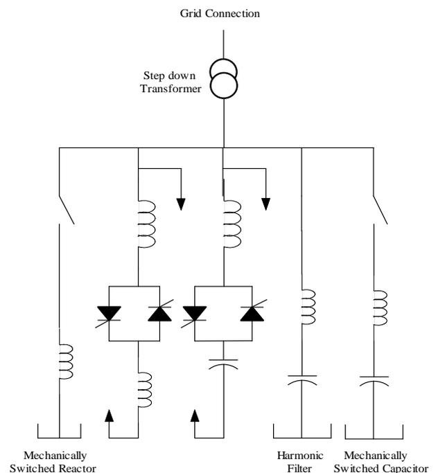
Fig. 10. Block Diagram of SVC
