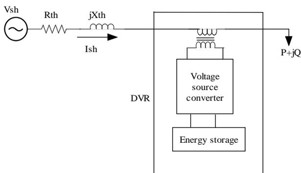
Fig. 9. Block Diagram of DVR
