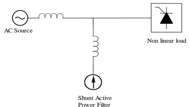
Fig. 8. Shunt Active Filter
