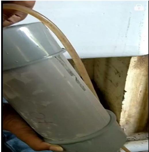
Fig. 2. Closing both sides with PVC caps
