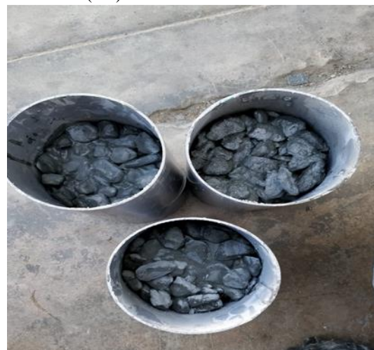
Fig. 1. Casting pervious concrete in PVC pipes
