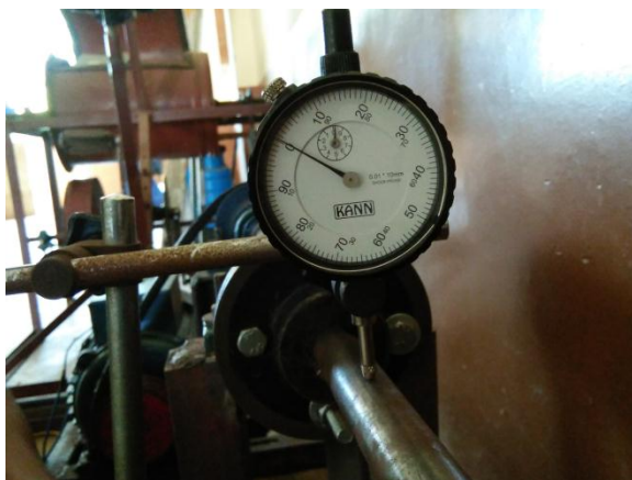
Fig.3.Checking Linearity of Shaft
