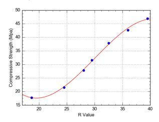
Fig. 2. Third Degree Polynomial Fit  $S = -0.0064R^3 + 0.57R^2 - 15.1R + 141.3$
